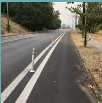
**Description:** A bicycle lane with a striped buffer area that separates the vehicular travel lane and the shoulder used for the bicycle lane.
