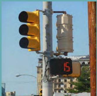
**Description:** Signal timings for pedestrians can include a leading pedestrian interval, which gives pedestrians a head start when entering an intersection. This enables pedestrians to establish their presence and enhances pedestrian visibility.
