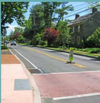
**Description:** Special paving treatments for crosswalks, which can include brick/pavers, colored or stamped asphalt, or thermoplastic pavement markings. Decorative crosswalks can be designed to reflect the unique character or identity of an area or neighborhood.
