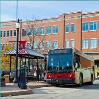
**Description:** Area adjacent and separate from the travel lanes on a roadway that provides space for buses to pick-up or drop-off passengers without impeding the flow of traffic. Bus bays are typically used on roadways with higher traffic volumes, higher speeds, or on congested corridors. They are also typically used for bus stops with higher ridership.
