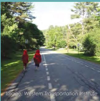
**Description:** A delineated, but nonexclusive space available for walking and biking on a roadway that is otherwise too narrow for other dedicated facilities. Area for walking and biking is identified with signage and pavement markings, typically a dashed white line 5 feet from the edge of the pavement on both sides of the roadway.
