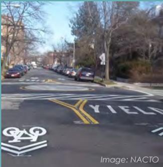
**Description:** Design treatments to offer priority for bicyclists operating within a roadway shared with motor vehicle traffic. Pavement markings, such as sharrows, and signage make users aware of the priority for bicycle travel and provide wayfinding. Can include traffic calming, access management, and other strategies to create a safe and low-stress environment for biking.
