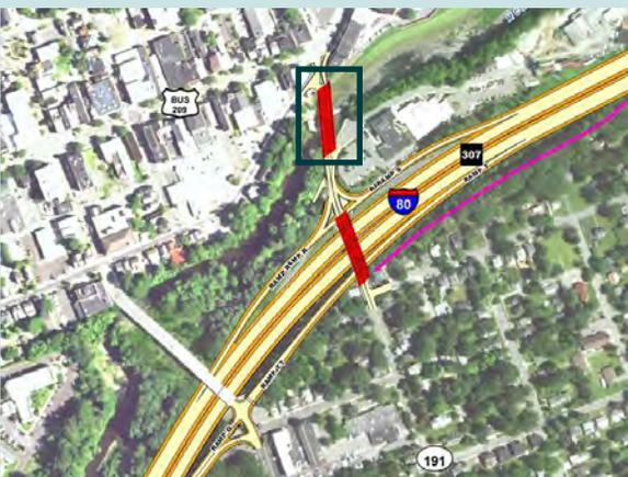
The Conceptual Plan for the I-80 Reconstruction, Phase II Alternative 2D, (Draft 2018) prepared by PennDOT, FHWA, and AECOM and posted on [i80project.com](http://i80project.com) includes replacement of the Broad Street Bridge over McMichael Creek. The draft conceptual plan includes sidewalks and bike lanes on both sides of the bridge. Additional design treatments, such as a barrier between along the curb, may be needed to create the gateway pedestrian connection to the Levee Loop Trail—South.
