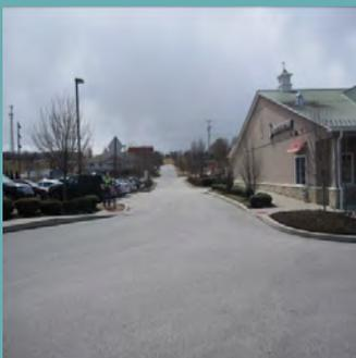
**Description:** Providing joint or cross access between adjacent properties allows circulation between the properties and reduces the number of driveways and conflict areas along a roadway. Joint and cross access can be used in combination with shared parking.
