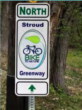
**Description:** Signs that can stand alone or mounted on an existing pole that identify a facility and provide directional information, particularly at key decision points. These signs are often used for on-road bicycle routes because they can be viewed by trail users and motorists.
