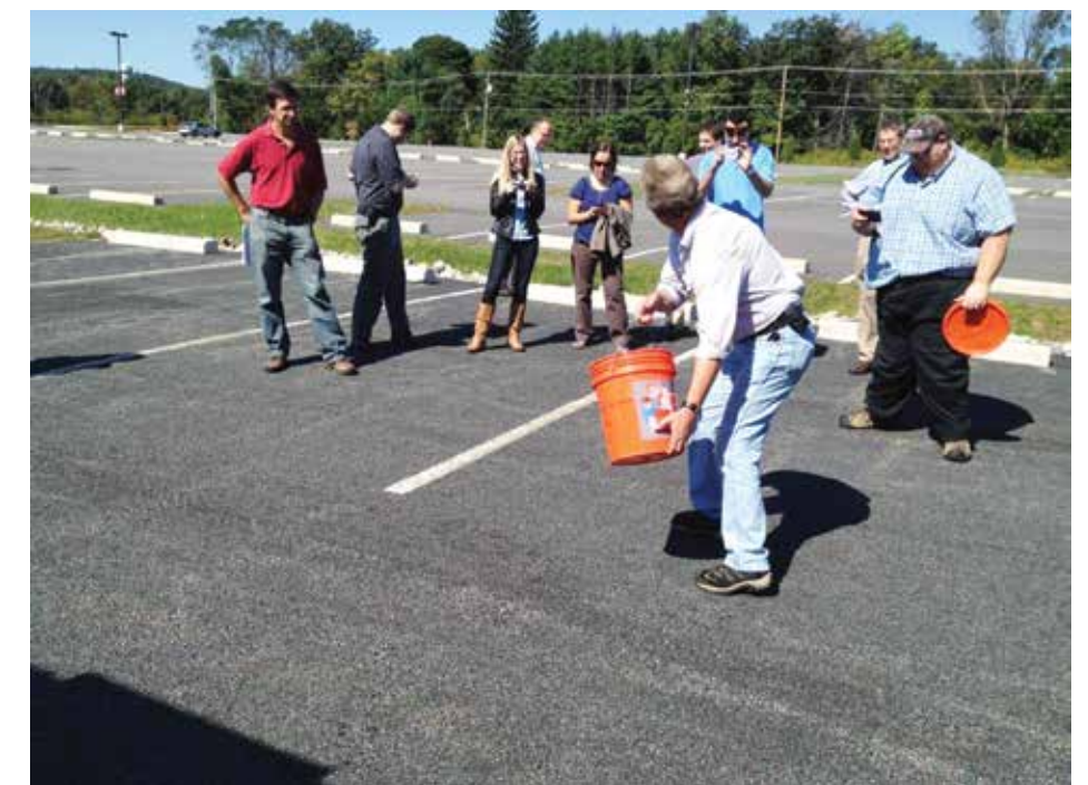
Demonstration of stormwater infiltration on permeable pavement
